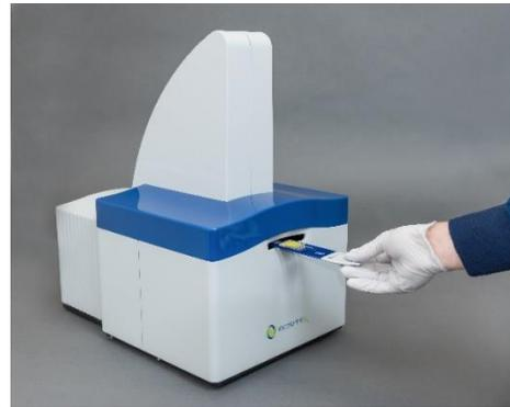
Figure 1. Shahky desktop instrument with consumable being inserted
